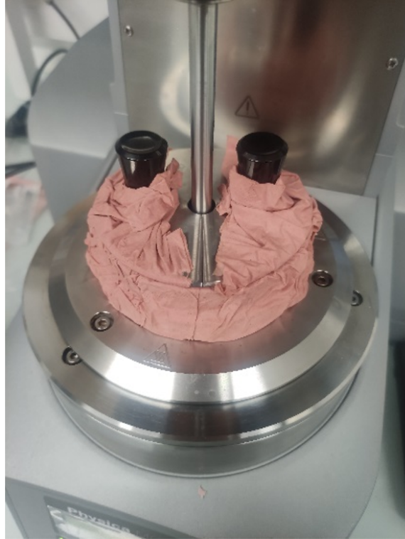
FIGURE IV.11 – Photography of the rheometer. The measurement is done inside the cage enveloped in wet paper to prevent evaporation.
