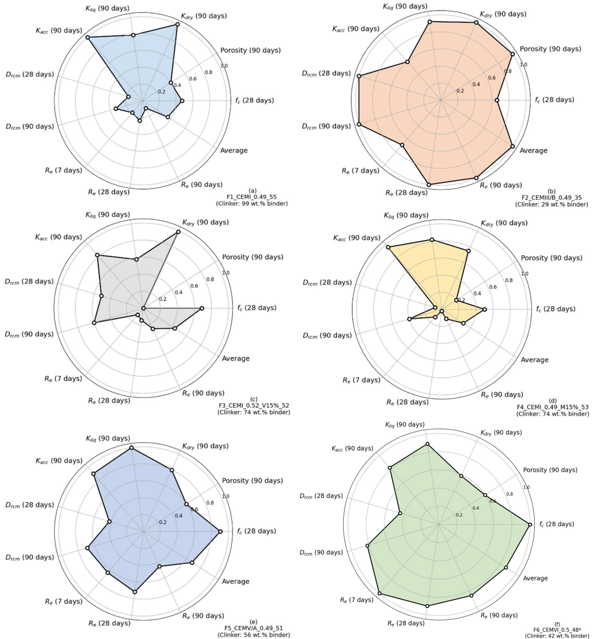
Figure II-40 Ratio of relative differences between MC and DC compared to the maximum obtained on the six formulations for F1 (a), F2 (b), F3 (c), F4 (d), F5 (e) and F6 (f).
