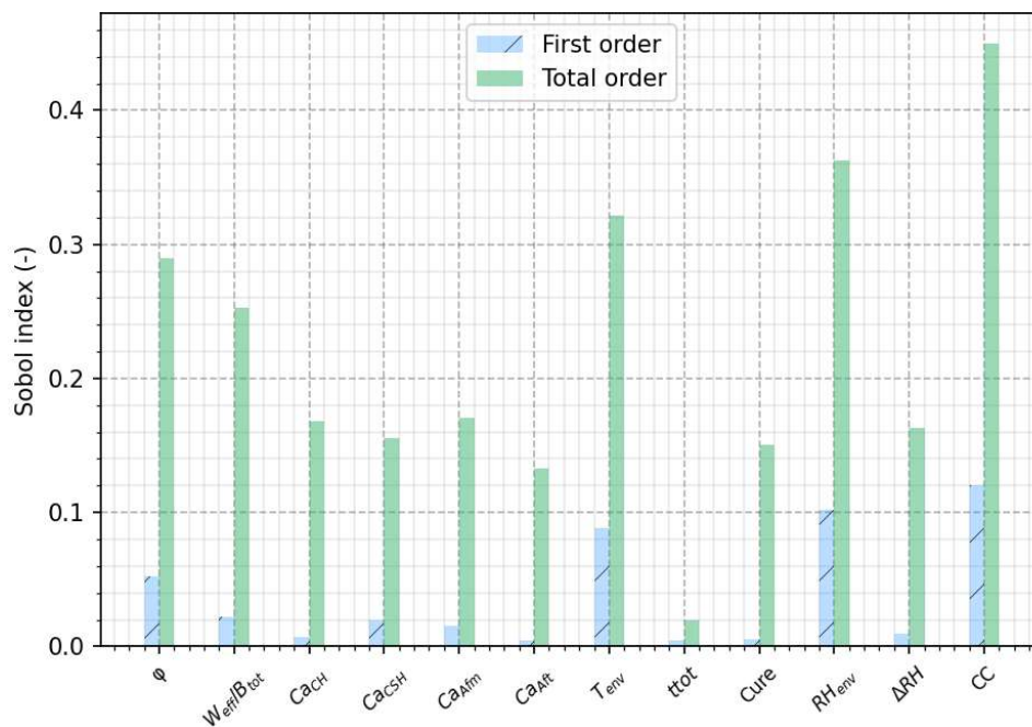
Figure III-38 First and total Sobol indices obtained for the surrogate model used for the saturation computation.
