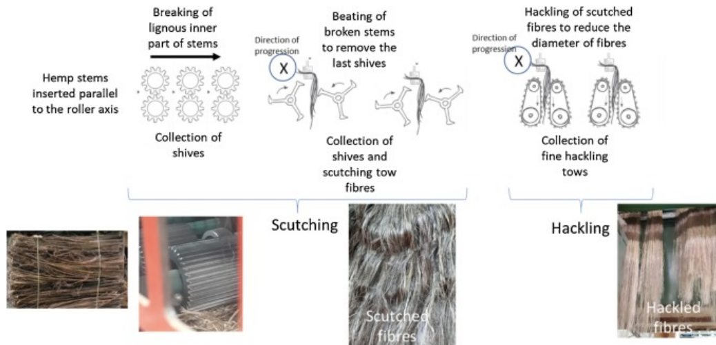
Figure 1.12: Scutching and hackling procedure for hemp fibers. Figure taken from [Grégoire 21] rearranged from [Müssig 15].
