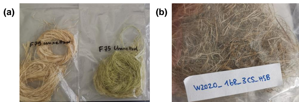
Figure 4.8: Examples of processed fibers from which bundles are extracted for peeling tests : (a) long strand, (b) short strand.
