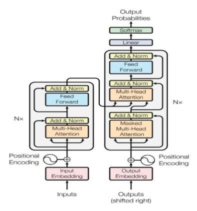
Figure 2.5: Transformers architecture. Source: [73]
