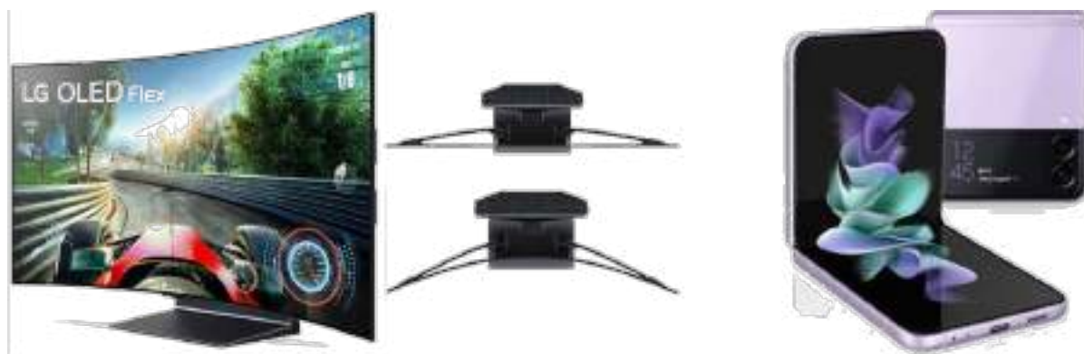
Figure 3.1 LG OLED flexible television (left) and foldable Samsung smartphone Galaxy Z Flip 3 (right).
