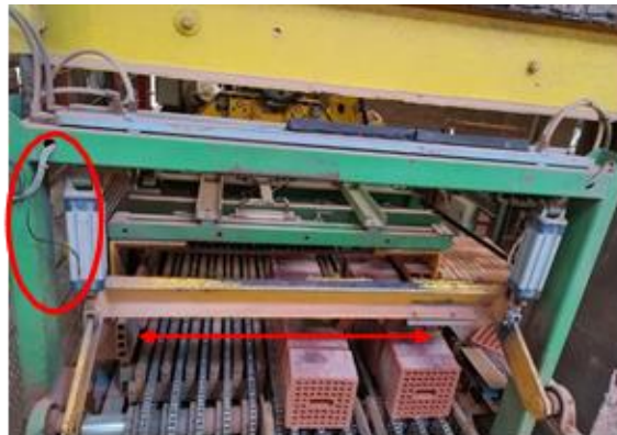
Figure 2.6. The location of the installed sensors
