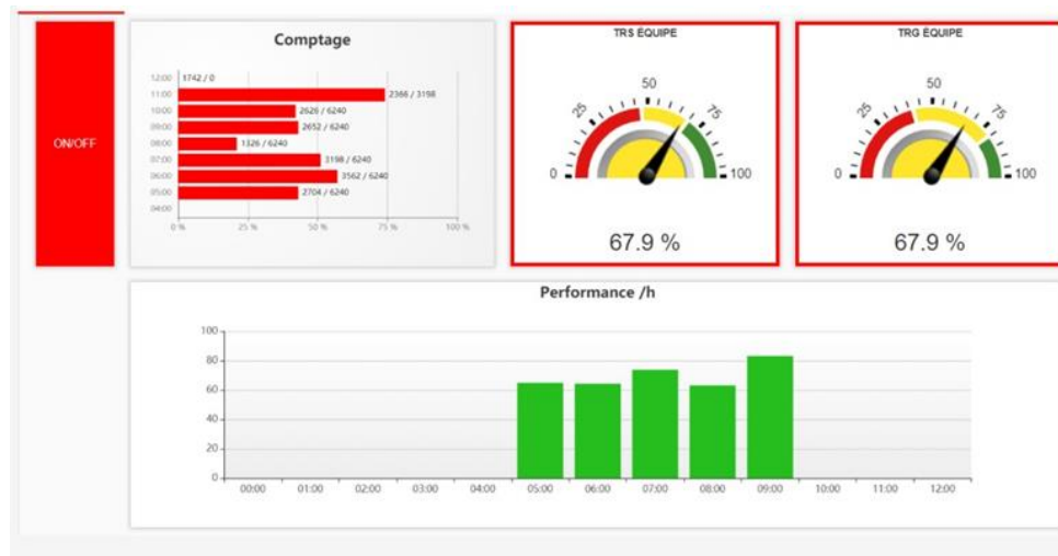
Figure 2.8. IoT Platform interface- Performance assessment and product counting
