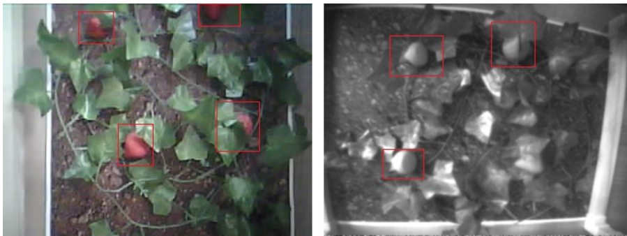
Figure 3.16: Image data acquired through the Arduino Portenta are on the right, and through the ESP32 cam are on the left
