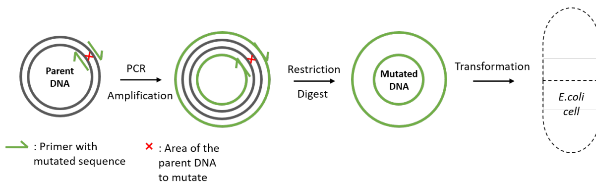
Figure 35 : Schematic of the site-directed mutagenesis procedure. The parent DNA is the DNA where the nucleotide sequence of interest is present (red cross). The amplification by polymerase chain reaction adds nucleotides on each side of the primers, by copying the nucleotide sequence of the parent DNA. The digest step removes the parent DNA, and the transformation step inserts the mutated DNA into a competent cell.
