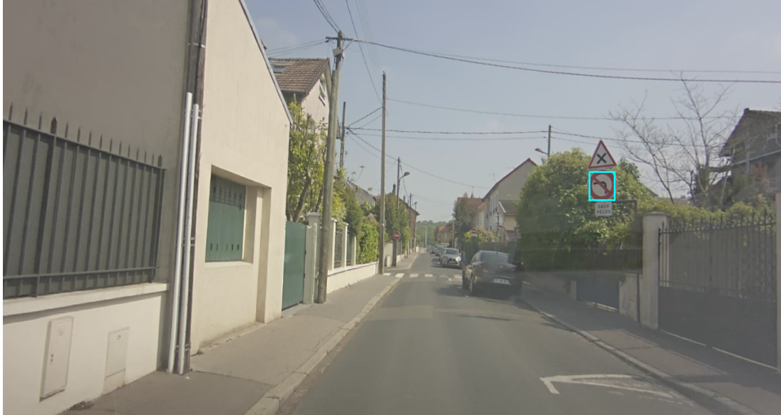
Figure 2.5: Detection of a traffic sign within an image issued by the monocular camera installed on our test-vehicle.
