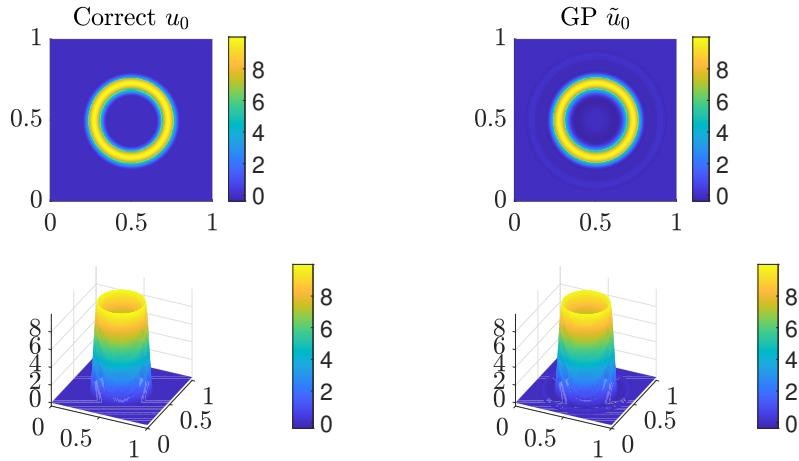
(b) Test case #1: True  $u_0$  (left column) vs WIGPR  $\tilde{u}_0$  (right column). 15 sensors were used. The images correspond to the 3D functions evaluated at  $z = 0.5$ .
