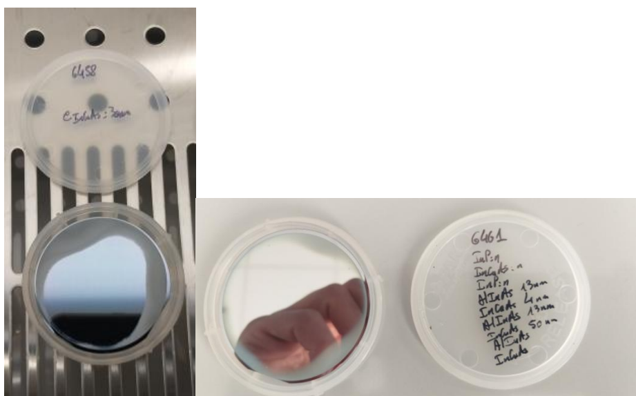
Fig. 4-14: Pictures of Sample HCSC-Barrier (on the left) and Sample HCSC-SQW (on the right) taken just after the MBE growth.
