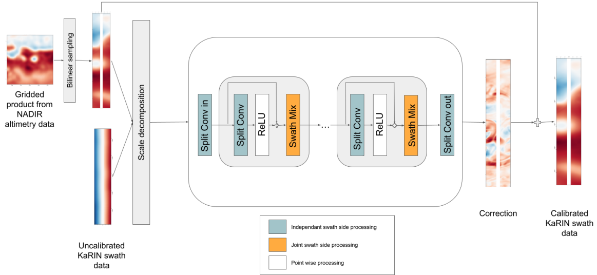
Figure 3.3 – Overview of the proposed architecture: From left to right: The first step interpolates the nadir-based gridded product onto the swath segment. Afterwards, both the nadir-based gridded product and KaRIn observation undergo the scale-space decomposition scheme outlined in 3.4. The scale components are stacked as channels and processed through the neural network. The blue color of the "Split Conv" indicates that each side of the swath is processed independently by the convolution layer whereas the orange coloring of the "Swath Mix" layer tells that the whole data is processed jointly (more details in 3.4). The final convolution computes a correction to be added to the gridded product for computing the calibrated KaRIn data
