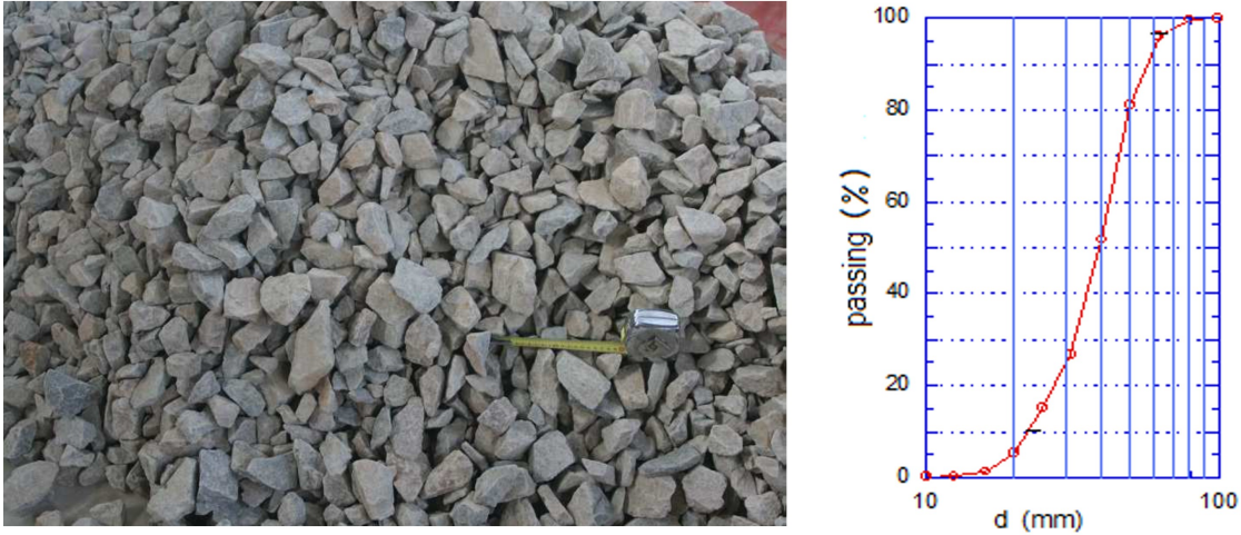
Fig. II.7. The rockfill used in PEDRA experimental campaign in addition to its particle size distribution curve
