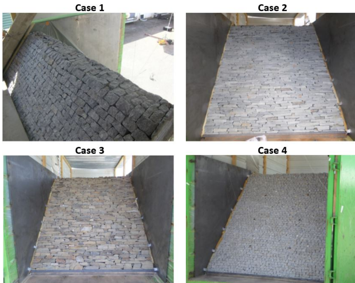
Fig. I.29. Dry-stone pitching of the four physical models in PEDRA experimental campaign
