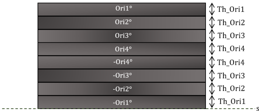
Figure 4.10: Illustration of the general composite laminate definition.
