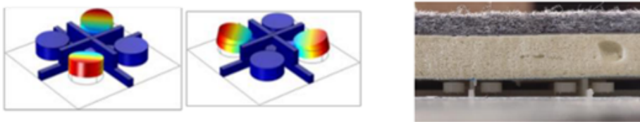
Figure 1.19: Considered small-scale resonators in [30] (left); Sound insulation pad with metamaterial layer (right) [30].
