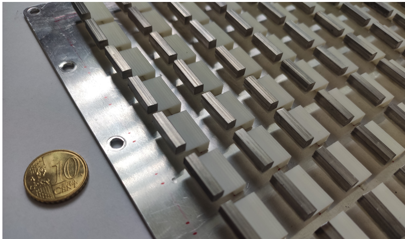
Figure 3.27: Close-up view of the LRM Plate (aluminium plate with 72 ABS-Steel micro-resonators) next to a 10 cent euro coin (for scale perception).
