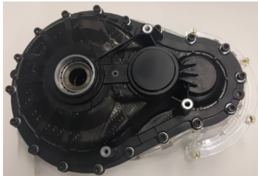
Figure 1.4: Composite gearbox housing by Schneider et al. [151].
