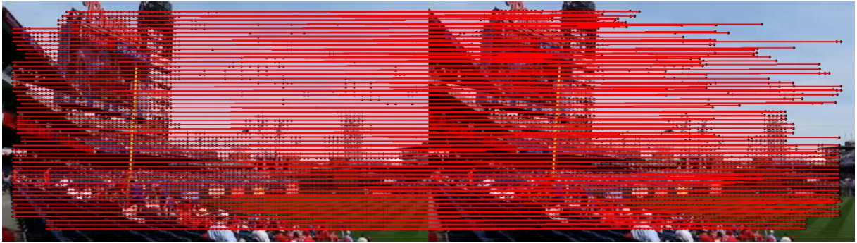
Figure 5.8. Correspondence between interest points in two successive frames.
