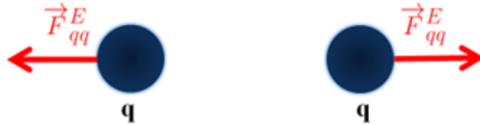
Figure 1.4 – Schematics of the Coulomb interaction between two particles of same charge q .
