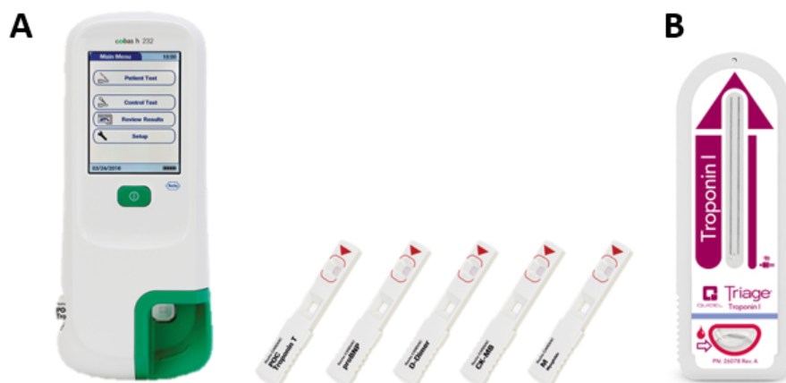
Figure 1.32: Examples of Lateral Flow Assays. (A) Roche Cobas h232 [31]. (B) Quidel Triage Cardiac
