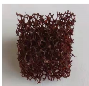
Figure 14. Photograph of the spent EY-APTES@PDA@PUF foam after six cycles of 2-methyl-5-nitro-isoquinolin-2-ium iodide oxidation.
