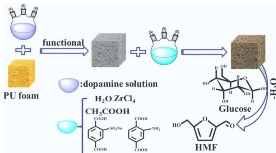
Figure 24. Preparation of acid-base bi-functional metal-organic frameworks membranes supported on PDA@PUF and their catalytic application (reproduced from ref. 130).
