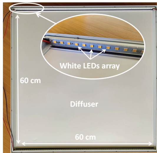
Figure 3.6 Typical LED light fixture used for indoor illumination (Sylvania START Panel Flat UGR19 600x600 Neutral White) consisting of 144 total mid-power LEDs and providing a luminous flux of 3500 lm.
