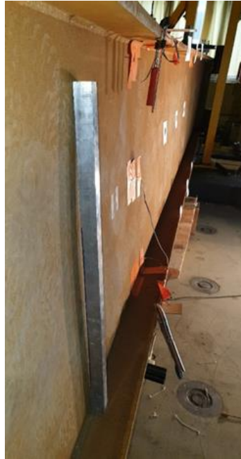
Figure VI-13: Post-peak web distortion in U-MS
