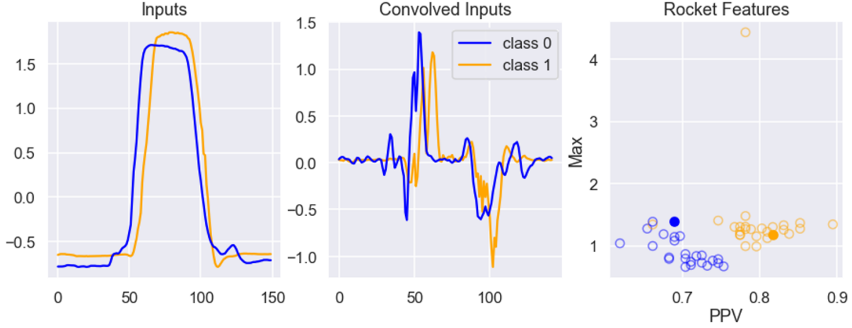
Figure 2.5: The different steps of the ROCKET method: first, transformation of the inputs using convolutional kernels, and then feature extraction from those convolved inputs
