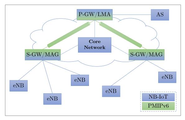
Figure 3.2: NB-IoT network architecture with PMIPv6.
