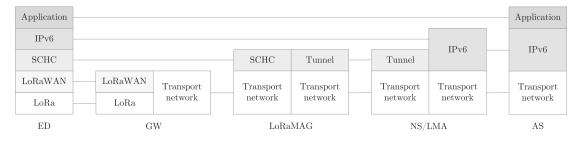
Figure 3.5: Evolved LoRaWAN user-plane protocol stack.
