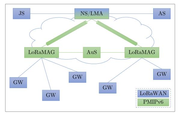
Figure 3.1: Evolved LoRaWAN architecture.
