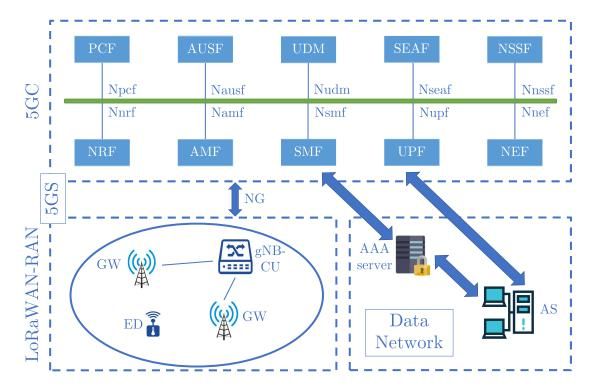
Figure 5.1: Proposed network architecture for integration.
