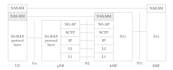
Figure 2.11: Control-plane protocol stack.
