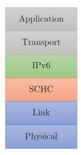
Figure 3.3: Mobile node protocol stack.
