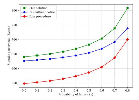
Figure 5.9: Variation of signaling overhead of access procedures in function of p.
