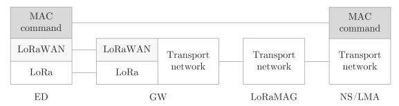
Figure 3.6: Evolved LoRaWAN control-plane protocol stack.
