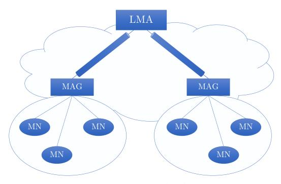
Figure 2.16: PMIPv6 network architecture.
