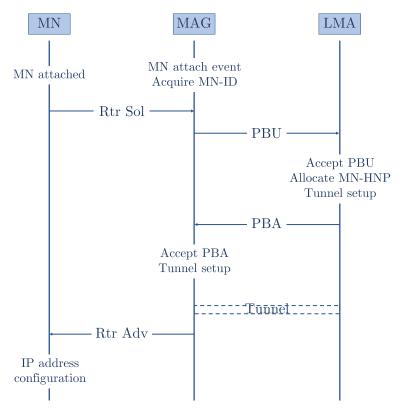
Figure 2.17: Mobile node attachment procedure.
