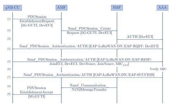
Figure 5.6: Secondary authentication using EAP-LoRaWAN-DN.
