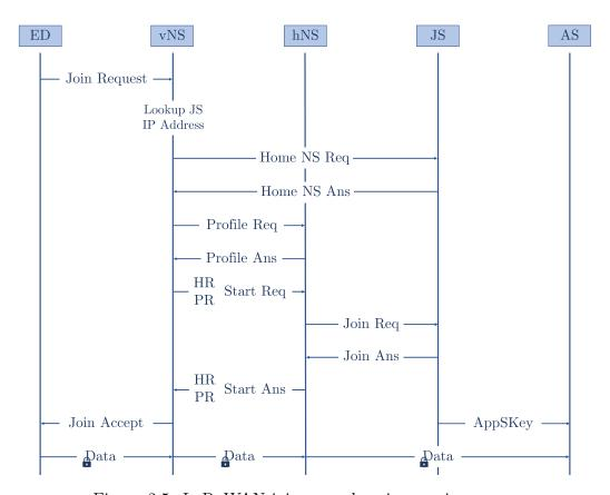
Figure 2.5: LoRaWAN join procedure in roaming cases.
