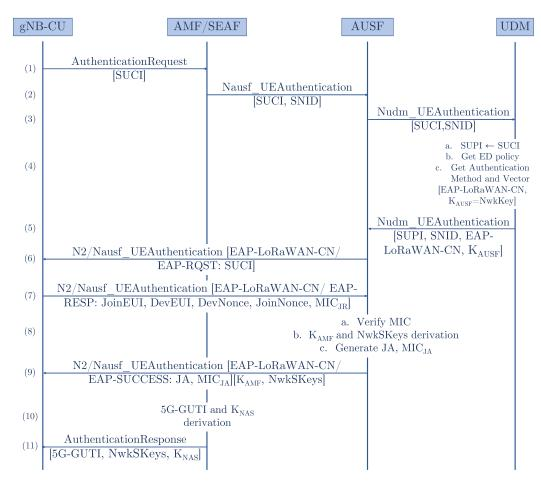
Figure 5.5: Primary authentication using EAP-LoRaWAN-CN.
