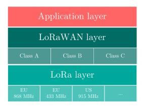
Figure 2.1: LoRaWAN protocol stack.
