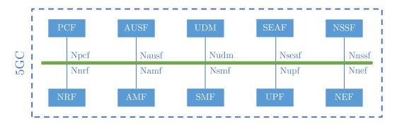
Figure 2.9: 5G core network functions.
