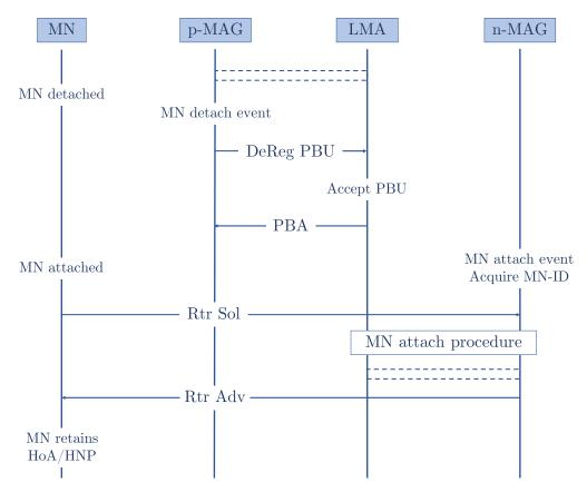
Figure 2.18: Mobile node handoff procedure.
