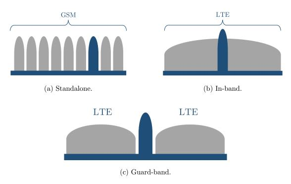
Figure 2.7: NB-IoT modes of operation.
