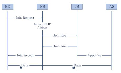
Figure 2.4: LoRaWAN join procedure in home network.
