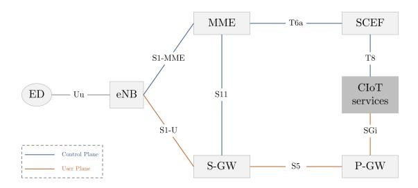
Figure 2.6: NB-IoT network architecture.
