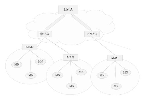
Figure 2.19: Cluster Sensor PMIPv6 network architecture.
