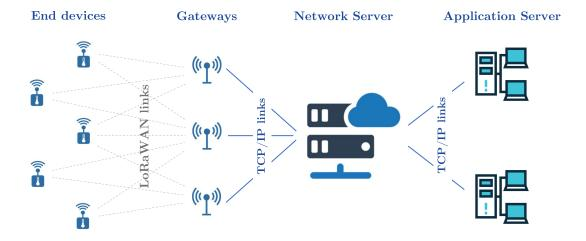
Figure 2.2: LoRaWAN network architecture.
