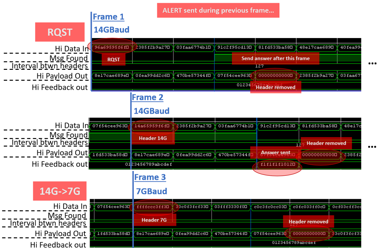
Figure 4.32 – Capture from the Deframer FPGA board showcasing a change of baudrate from 14GBaud to 7GBaud with the auto-negotiation protocol. The ALERT message was sent before the first pictured frame.
