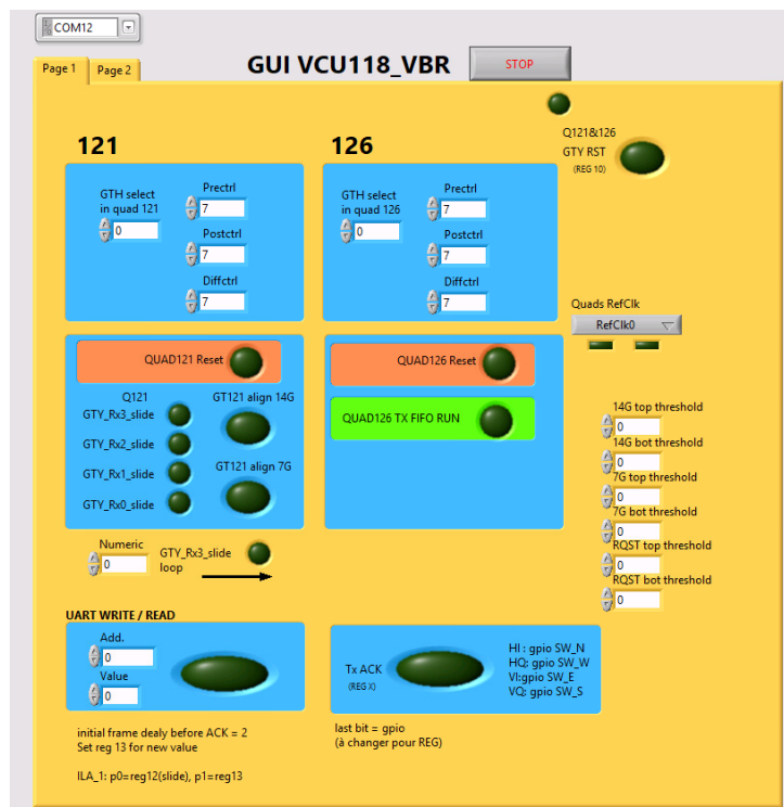
Figure 4.31 – Labview developed interface to pilot the deframer board, connected via UART.
