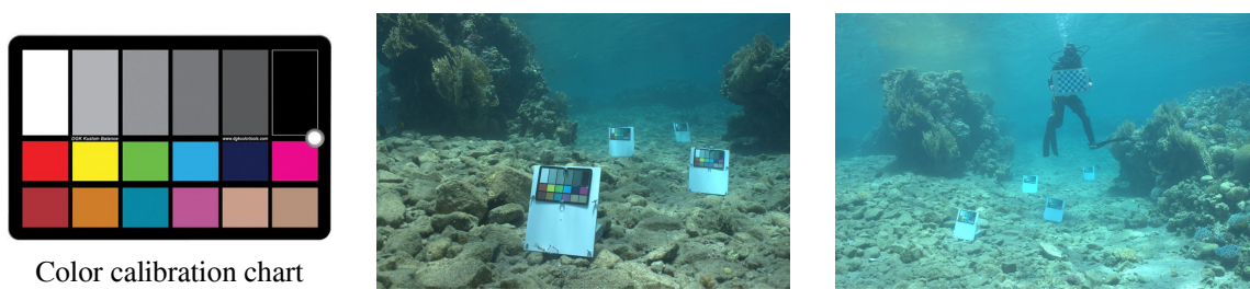
Figure 4.12: Sea-thru D5 dataset. The Sea-thru D5 dataset provides images in a raw file format with four color calibration charts dispatched across the scene.
