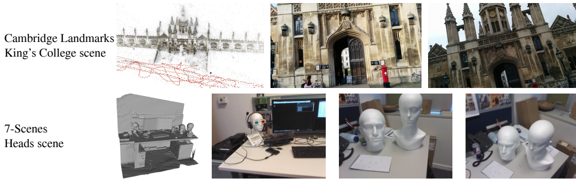
Figure 5.6: Cambridge Landmarks and 7-Scenes datasets. Cambridge Landmarks ground truth is obtained using SfM. 7-Scenes ground truth is obtained using RGB-D SLAM.
