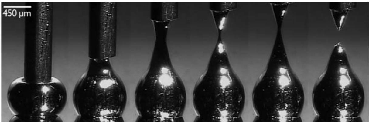
Figure I–18 A series of photographs of the formation of a conical tip of EGaIn [84].
