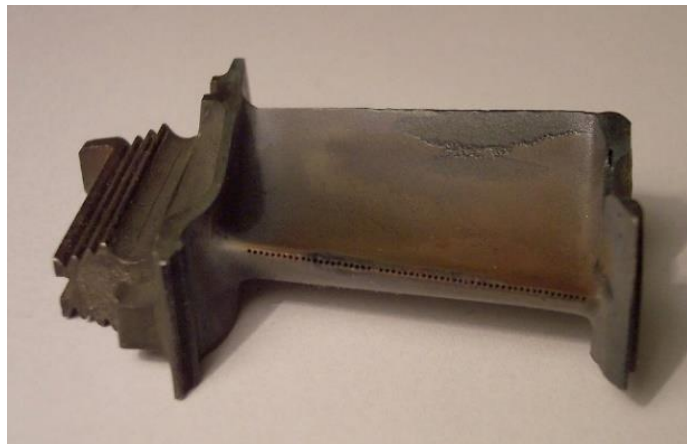
Figure 9. Turbine blade from a Turbo-Union jet engine [28].
