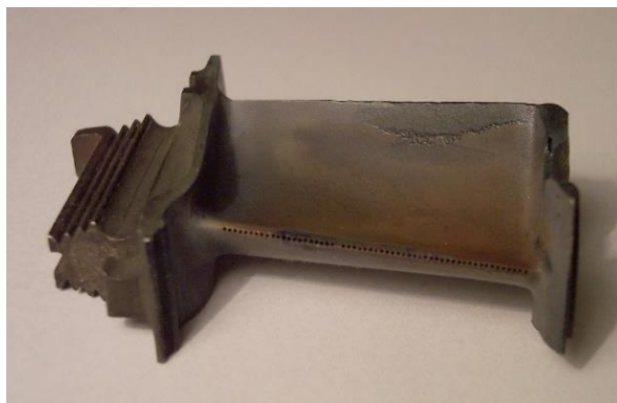
Figure 9. Turbine blade from a Turbo-Union jet engine [28].
