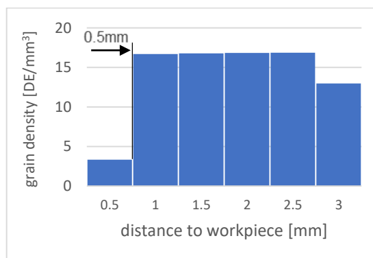
Figure 69. Surface grain density in \mu SM and R \mu SM. Boundary-induced lower density in the R \mu SM
