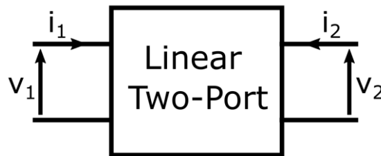
Figure C.3 Schematic of a linear two-port
