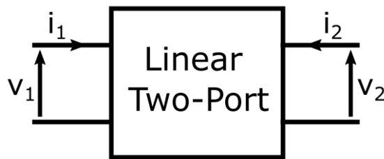
Figure 3.1 Schematic of a linear two-port
