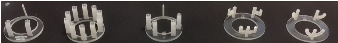
Figure 36 – Examples of exoskeletons made to improve the bare Kilobot and potentially generate effects on the dynamics. Exoskeletons differ by the multiplicity of their legs, as well as the position of the center of mass of the robot. Different types of resin were also tested. The two exoskeletons to the right were made to hold small toothbrush-like brushes, effectively changing the type of legs in contact with the ground.
