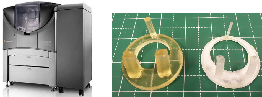
Figure 37 – Left The Stratays Connex3 Objet260 printer. This printer uses a photosensitive resin and UV light to achieve a precision up to 20\mu\text{m} . Printing one exoskeleton takes about 30 minutes, but as it does not require human monitoring, most of the printing is done overnight. Right The prints are first encapsulated in a support resin that needs to be scrapped out manually. The part is then rinsed and cleaned to achieve the final result.
