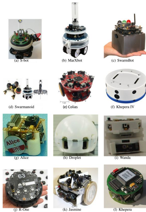
Figure 5 – Catalog of robots used in the swarm robotics literature, edited from Nedjah et al. 2019 [21].
