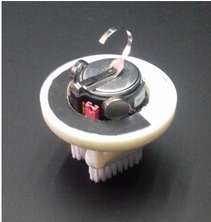
Figure 39 – Corner view of a Kilobot inside the toothbrush exoskeleton.
