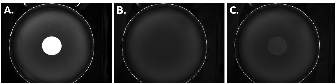
Figure 44 – Example images captured from the camera of the circular arena, exposure time 100ms, 4096x3000. A. No filter with green projection. (+12dB) B. Red filter (645nm) with green projection. (+24dB) C. Red filter (645nm) with red projection. (+24dB)
