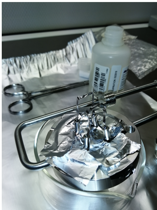
Figure 4.1: Tantalum filament mounted on the filament flange of the S 3 -LEB gas cell.
