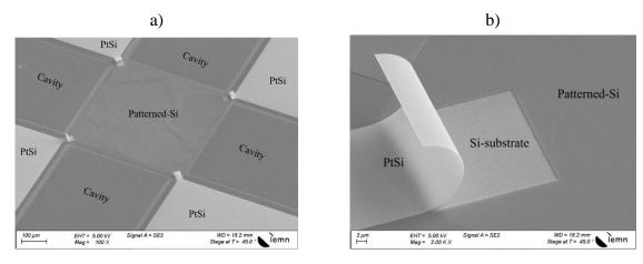
Figure 4-22: SEM images of a) Vander Pauw structures for patterned Si and b) a close-up view on the detached contact from the membrane.
