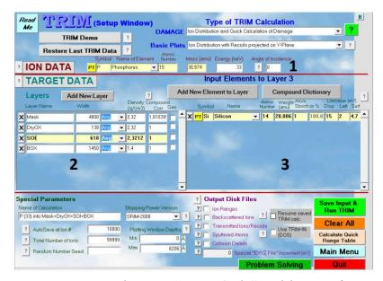
Figure 3-22: Ion implantation "Monte-Carlo" modeling interface.
