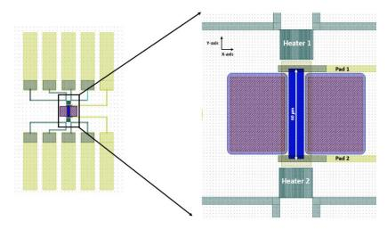
Figure 3-8: Seebeck coefficient measurement device.
