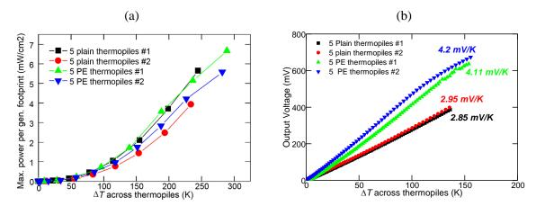
Figure 1-23: (a) Electric power generation per generator footprint of 2 samples of patterned thermopiles (PE) and 2 samples of plain membranes(plain) as a function of the temperature difference across the thermopiles; (b) The output voltage and the Seebeck coefficient of 2 samples of patterned thermopiles (PE) and 2 samples of plain membranes(plain) as a function of the temperature difference across the thermopiles[1].
