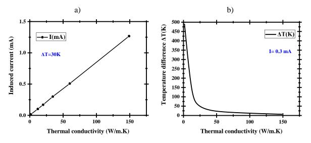
Figure 2-22: Calibration curves: (a) Current vs. thermal conductivity at 30K temperature difference, and (b) Thermal conductivity vs. temperature difference across the membrane (70nm thickness, 10μm width, 60μm length).
