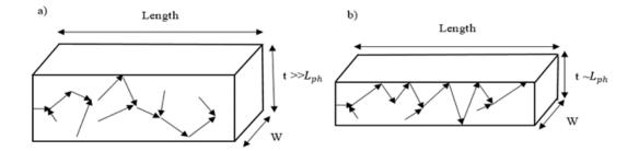
Figure 1-7: Phonon propagation in the material, a) in bulk material, b) in nanostructured material.
