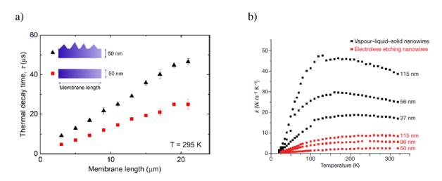
Figure 1-13:(a) Thermal decay time as a function of length of 50 nm-thick silicon membranes with and without nano-cones at 295K[32], (b) Thermal conductivity of rough Si nanowire (black lines) with different diameters and smooth one (red lines) as a function of temperature[44].
