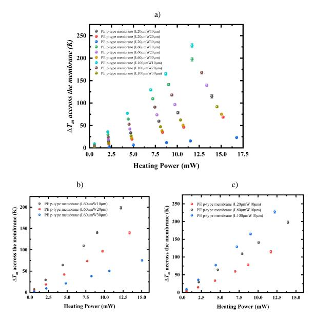
Figure 4-7: The temperature difference across p type silicon PE membranes with a) with different length and width ranging from 20 μm to 100 μm for length and 10 μm to 30 μm for width b) varying widths but the same length 60μm, b) different lengths but the same width 10μm.
