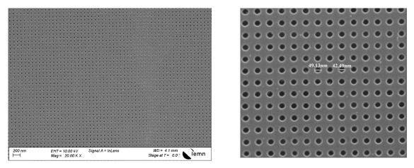
Figure 4-28: Scanning Electron Microscopy image of periodic patterned nano-holes in silicon.
