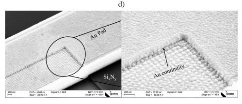
Figure 3-34: SEM images after gold evaporation for a) zT figure of merit direct measurement device, b) Close up view of zT direct measurement device, c) Seebeck measurement device and d) close up view of Au/PtSi contact.
