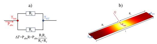
Figure 4-29: a) Electrical analogy of two thermal resistors that corresponds to the right and left paths. b) Plain Si membrane in the form of a slab with spots of laser heating at the center and room temperature heat-sink at the ends.
