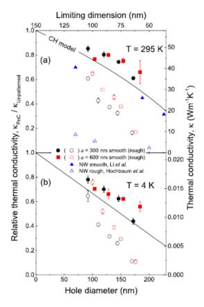
Figure 1-15:Measured thermal conductivity of 1D PnCs and nanowires (NWs) as a functions of the hole diameter and the limiting dimension (neck size) at (a) T=295K and (b) T=4K for pitch a=300 nm (black circles) and a=600 nm (red circles)[49].
