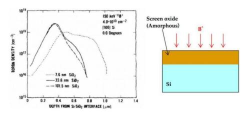
Figure 3-19: Boron dopant profile with various screen oxide thickness [83].
