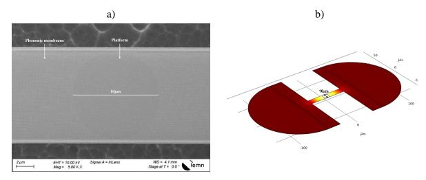
Figure 4-34: a) Scanning Electron Microscopy (SEM) image of a fabricated 60nm-thick Si Phononic membrane with a 100nm pitch and a plain 10µm diameter platform positioned at the center of the membrane. b) Finite Element Modeling (FEM) representation of the patterned membranes with an unpatterned diameter at the center (HPE) device, illustrating the contour of the platform.
