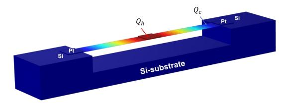
Figure 2-9: Schematic of zT direct measurement device adapted to membranes using Harman technique. When a DC current passes through the membrane, Peltier heating  $(Q_h)$  and Peltier cooling  $(Q_c)$  occur at each membrane extremity and heat flow through the membrane  $(Q_{Heat})$ .
