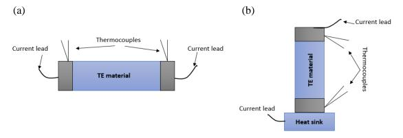
Figure 2-1: Harman's method principle (a) without heat sink; (b) with heat sink.
