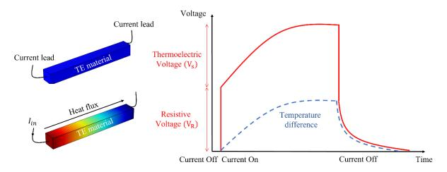
Figure 2-2: Schematic of Harman measurement method depicting i) the suspended thermoelectric element before and after injection of a DC current  $I_{in}$  ii) the measured voltage accross the sample versus time.
