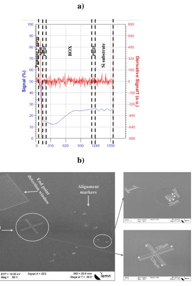
Figure 3-13: a) The end point detection signal (blue) and its derivative (red), b) SEM images of the etched alignment markers, end point detection window and the alignment cross.
