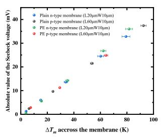
Figure 4-9: The absolute measured Seebeck voltage as a function of the temperature difference across different Si membranes. The data points represent different membrane types: phononic-engineered (PE) p-type membrane is represented in red, plain p-type membrane in black, plain n-type membrane in blue, and PE n-type membrane in green.
