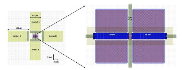
Figure 3-6: Design of transient Harman measurement platform.
