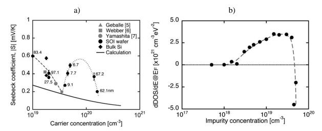
Figure 4-12:a) Absolute Seebeck coefficient of SOI wafers as a function of carrier concentration. The solid line represents the calculated value, and the broken and the dotted lines are drawn as an eyeguide. b) Energy derivative of DOS at the Fermi energy, computed on the basis of the three influences of the heavy doping, as a function of impurity concentration. The broken line is drawn as an eye-guide [91].
