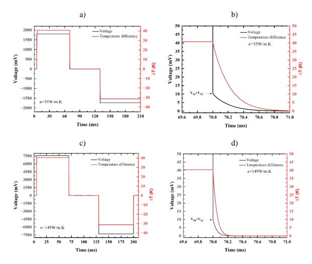
Figure 2-20: (a,c) Voltage and temperature profiles for different thermal conductivities. (b,d) A close-up of the cooling slope and Seebeck voltage for different thermal conductivities.
