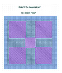
Figure 3-7: Van Der Pauw resistivity measurement device.
