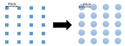
Figure 3-16: Overdosing methodology principle[81].
