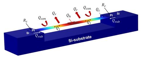
Figure 2-5: Schematic of zT direct measurement device adapted to membranes. When a DC current passes through the membrane, Joule heating  $(Q_J)$  raises the membrane's temperature. Heat flow from the membrane to the environment occurs via conduction through the anchors at the extremities  $(Q_{sub})$ , convection  $(Q_{con})$ , and radiation  $(Q_r)$ . With a DC current, Peltier heating  $(Q_h)$  and Peltier cooling  $(Q_c)$  occur at each membrane extremity.
