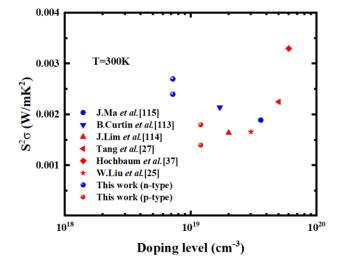
Figure 4-37: Power factor as a function of doping level. The graph includes experimental data from previous studies, as well as data from this current work, encompassing both n-type silicon (indicated in blue) and p-type silicon (represented in red) at a temperature of 300 K.
