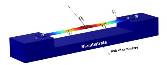
Figure 2-11: Schematic of zT direct measurement device adapted to membranes using Harman technique and considering the Joule heating effect. When a DC current passes through the membrane, Joule heating  $(Q_J)$  raises the membrane's temperature.), Peltier heating  $(Q_h)$  and Peltier cooling  $(Q_c)$  occur at each membrane extremity and the heat flows through the membrane  $(Q_{Heat})$ .
