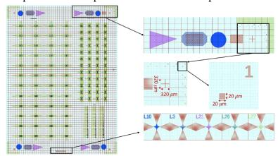
Figure 3-4: Cell containing transient Harman devices, Seebeck coefficient measurement devices and thermal conductivity measurement devices for a wide range of suspended planar silicon membrane geometries with a close-up view on the end point detection windows (top), alignment markers (middle) and alignment verification crosses (bottom).
