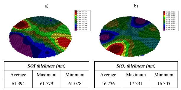
Figure 3-21: Full wafer SOI and SiO<sub>2</sub> thicknesses 49-point mapping highlighting the thickness dispersion a) SOI thickness mapping; b) SiO<sub>2</sub> thickness mapping.
