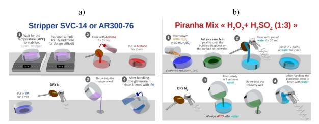
Figure 3-12: Wafers cleaning procedure a) Resist stripping, b) Piranha process<sup>4</sup>.
