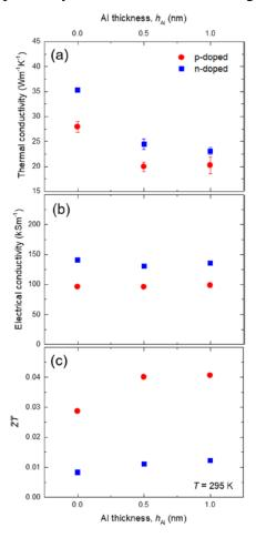
Figure 1-11: Measured (a) thermal conductivity, (b) electrical conductivity, and (c) figure of merit (zT) of Si membrane as a function of aluminum set thickness[45].
