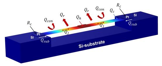
Figure 2-13: Schematic of zT direct measurement device adapted to membranes. When a DC current passes through the membrane, Joule heating  $(Q_J)$  raises the membrane's temperature. Heat flow from the membrane to the environment occurs via conduction through the anchors at the extremities  $(Q_{sub})$ , convection  $(Q_{con})$ , and radiation  $(Q_r)$ . With a DC current, Peltier heating  $(Q_h)$  and Peltier cooling  $(Q_c)$  occur at each membrane extremity.
