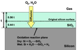
Figure 3-20: The basic process for the oxidation of silicon [84].
