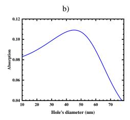
Figure 4-27: RCWA absorption coefficient as a function of (a) thickness of plain membranes and (b) hole's diameter of a 60nm thick patterned membrane with a 100nm pitch. The calculations are based on the refractive index obtained from Palik (n=4.463+ i\*0.0367).
