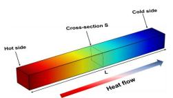
Figure 2-6: Thermal conduction.
