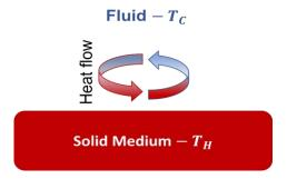
Figure 2-7: Thermal conducto-convection transfer.
