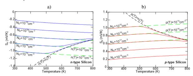
Figure 1-5: Silicon Seebeck coefficient versus temperature for different doping concentrations. Blue continuous line for n-type doping. Red continuous line for p-type doping. Green dashed line assuming carrier and doping concentrations equality and temperature independence. Black dashed line Seebeck coefficient in intrinsic semiconductor <sup>2</sup>.
