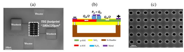
Figure 1-22: (a)  $\mu$ TEG made of 5 suspended thermopiles; (b) Cross section of the  $\mu$ TEG giving the heat flow direction; (c) Opening of a network of "pores" of ~ 40nm in diameter and spaced 100nm ("pitch")[1]
