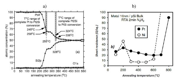
Figure 3-31: a) Platinum silicide formation mechanism and kinetic [85] and b) PtSi sheet resistance with respect to the annealing temperature [86].
