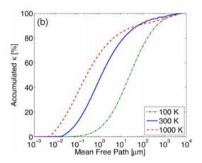
Figure 1-6: Accumulated silicon κ over wide range of phonon's free path for different temperatures[23].
