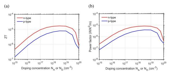
Figure 1-3: (a) Si zT as a function of doping concentration, (b) Si power factor as a function of doping level; blue line refers to p-type Si and red line to n-type Si<sup>1</sup>.
