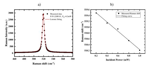
Figure 4-25: a) the characteristic Lorentz distributions obtained from measurements on a plain p-type Si membrane with dimensions of  $20\mu m$  in length and  $10\mu m$  in width for an incident power levels equal to 0.2mW. b) Variation of Raman shift as a function of the incident power of a p-type plain membrane, t=60nm,  $L=20\mu m$ ,  $W=10\mu m$ .
