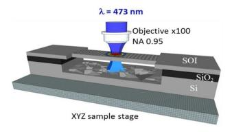
Figure 4-23: Schematic representation of the phononic membrane measurement process of the  $\mu RT$  experiment utilizing one laser source[106]<sup>5</sup>.
