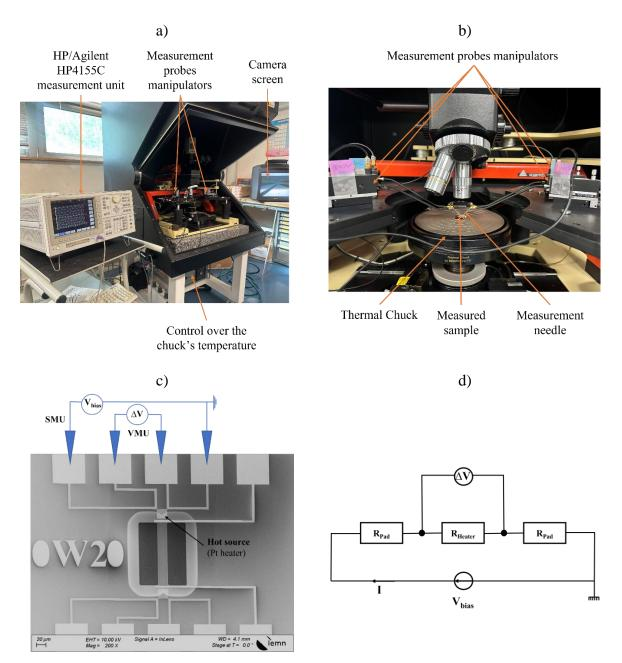
Figure 4-3: Pt heater calibration. (a) Measurement platform showcasing the setup used for characterizations. (b) Close-up view of the measurement set-up. (c) Probes' positioning in the Seebeck coefficient measurement device. (d) Electrical circuit analogy of the Pt heater calibration.
