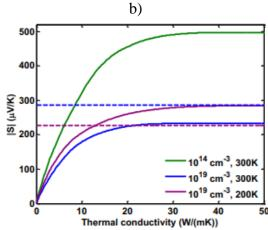
Figure 4-15: a) Phonon mode-specific accumulated contributions to the phonon drag Seebeck coefficient and the thermal conductivity with respect phonon mean free path. Solid lines show the contribution at 300 K, and dashed lines are used at 200 K and dotted lines at 100 K. These results are obtained for lightly doped n-type silicon. b) Contribution of the most preferable modes to the phonon drag Seebeck coefficient at different reduced thermal conductivity values [87].
