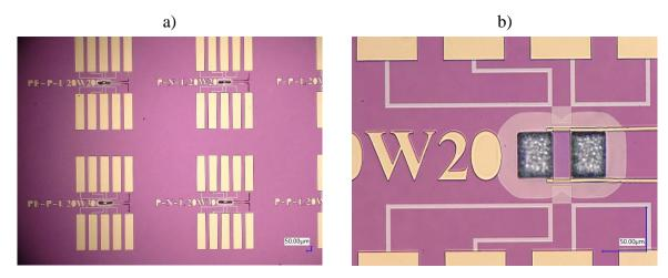
Figure 3: The microscope images showcase a) the fabricated Seebeck coefficient measurement device, b) a close-up view of the Si suspended membrane within the Seebeck coefficient measurement device.
