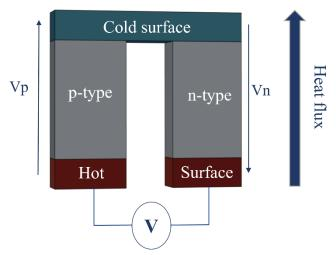
Figure 1-2: Thermoelectric power generating device principle.
