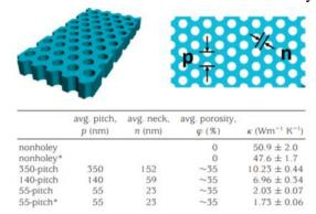
Figure 1-14: Holey silicon geometry and the measured thermal conductivity at 300K, \*denotes doped samples (Boron  $(5.10^{19} \text{ cm}^{-3})[52]$ .
