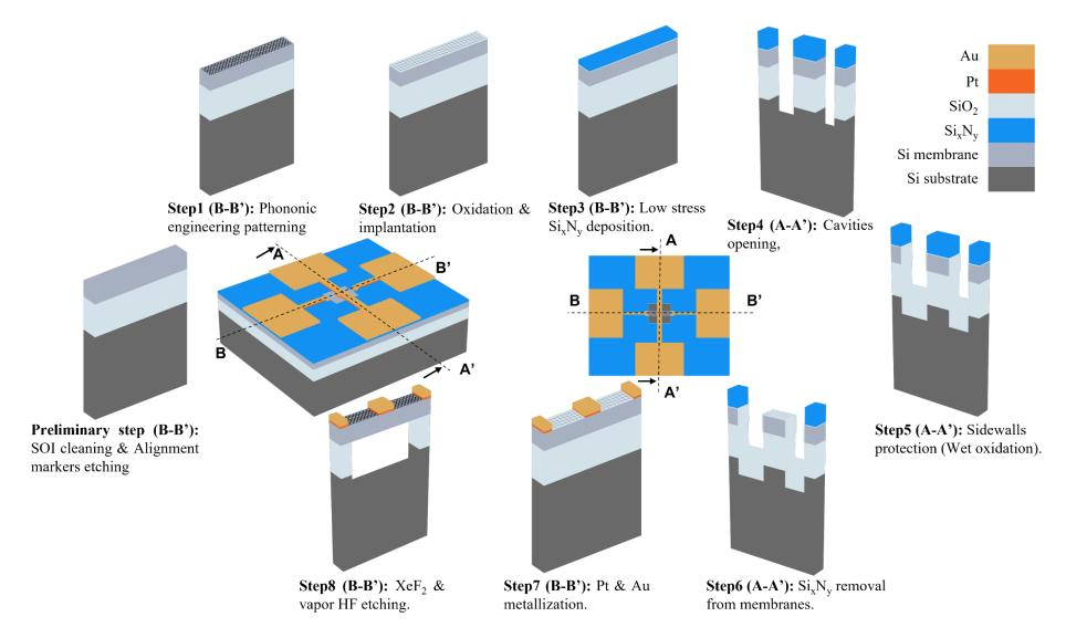
Figure 3-11: Fabrication process steps.
