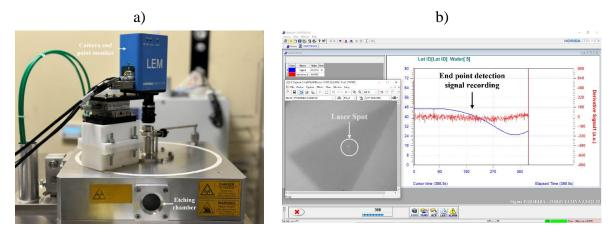
Figure 3-5: a) Camera end point monitor mounted on the dry etching chamber, b) Laser spot and the end point detection signal recording.
