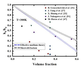
Figure 1-17: The thermal conductivity of silicon phononic crystals  $(\kappa_h)$  /the thermal conductivity of plain silicon  $(\kappa_p)$  ratio at 300K as a function of volume fraction, including the effective medium theory (blue circles) and Maxwell-Eucken (black circles) fitting.
