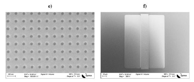
Figure 3-30: a) End point detection signal of SixNy removal step from membrane, SEM images of b) alignment cross marker of layer 21, c) SixNy removal from Si membranes in direct zT measurement device, d) close-up view of patterned Si membrane, e) patterns in Si membrane and f) SixNy removal from Si membranes in Seebeck coefficient measurements device.
