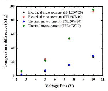
Figure 4-18: Temperature difference as a function of voltage bias for PNL20W20 and PPL60W10 Samples: Comparison of electrical and thermal measurement techniques.
