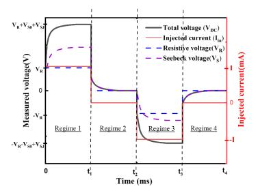
Figure 2-12:  $V_{s0}$  extraction method using two opposite values of injected current. Injected current in the system (red line), measured total voltage  $(V_{DC})$  across membranes (black line), measured Seebeck voltage  $(V_S)$  across membranes (purple dashed line), measured resistive voltage  $(V_R)$  across membranes (blue dashed line) are reported as a function of time.
