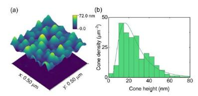
Figure 1-12: (a) AFM images of membranes with (upper) and without (lower) nanocones.(b) Histogram of nanocone height distribution [32].
