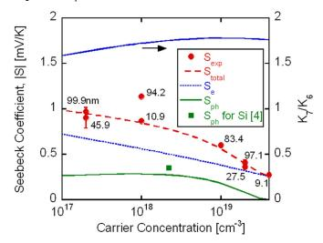
Figure 4-11: (Left y-axis) S and (right y-axis) ratio of the parameter integral, as a function of carrier concentration. The broken, dotted, and solid lines represent  $S_{total}$ ,  $S_e$ , and  $S_{ph}$ , respectively. The filled square represents the reported  $S_{ph}$  value for bulk Si[92].
