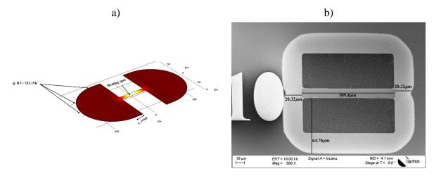
Figure 4-31: a) COMSOL model for thermal conductivity fitting using experiment geometry and Finite Element Model analyses for heat transfer. b) Scanning Electron Microscopy image of the suspended membrane, showcasing the width of the created wings.
