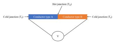
Figure 1-1: Principle of a thermocouple, illustrating the thermoelectric effect. The voltage (V) generated is proportional to the temperature difference  $(T_H - T_0)$  between the hot junction  $(T_H)$  and the cold junction  $(T_0)$ .
