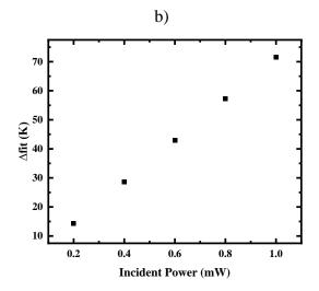
Figure 4-26:a) From Balkanski et al. [108], Raman shift as a function of temperature. The solid and dashed curves are model fit accounting for free- and four-phonon and only free-phonon processes respectively. Thick line is a guide to the eye highlighting the idea of linear approximation between 300K and 800K. b) The experimental temperature difference across the p-type membrane with t=60nm, L=60µm and W=10µm as a function of the incident power.
