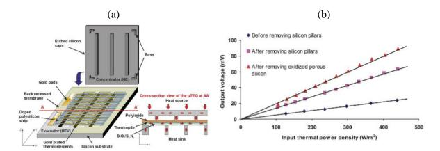
Figure 1-21: (a) 3D "exploded" structure and cross-section view of a 3-membranes planar  $\mu$ TEG. The red arrows symbolize heat paths; (b) Output voltage of the 5-membranes  $\mu$ TEG as a function of the input power density[57].
