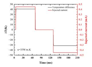
Figure 2-19: Temperature Difference and Injected Current at the center of the planar Si membranes (of length equal to 60µm, width equal to 10µm and thickness of 60nm) over Time in Nanostructured Si Membrane.
