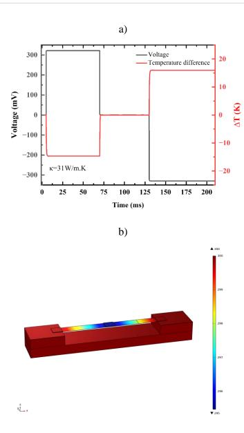
Figure 2-21: a) Measured Voltage and Temperature Profiles across the plain p-type membrane using the measured transport properties. b) Temperature profiles in the plain-p type membrane with an injected current equal to 0.1mA.
