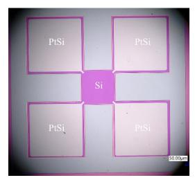
Figure 2: Microscope image of the fabricated Van Der Pauw structure, for the measurement of the electrical conductivity.
