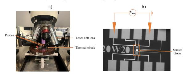
Figure 4-16: (a) Experimental Setup Configuration for Transient Thermo-Reflectance (TTR) Measurement. (b) A Reference Image via TTR, Demonstrating Probe Placement for Voltage Bias.
