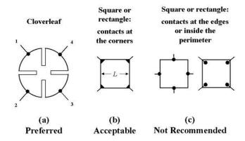
Figure 4-19: Samples' choice for VDP electrical conductivity measurements
