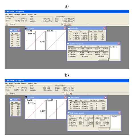
Figure 1: Electrical resistivity and carrier concentration of a 60nm plain membranes a) p-type, b) n-type.
