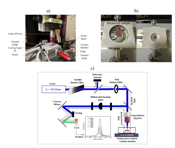
Figure 4-24: Experimental Setup for Micro Raman-Thermometry. a) The configuration of the experimental setup utilized for micro-Raman-thermometry. b) a close-up view of the measured sample within the vacuum chamber. c) a schematic of a Raman microscope analogous to LabRAM HR confocal system from Horiba Jobin-Yvon used with 473.11 nm continuous-wave diode-pumped laser (credited to Akash Patil).
