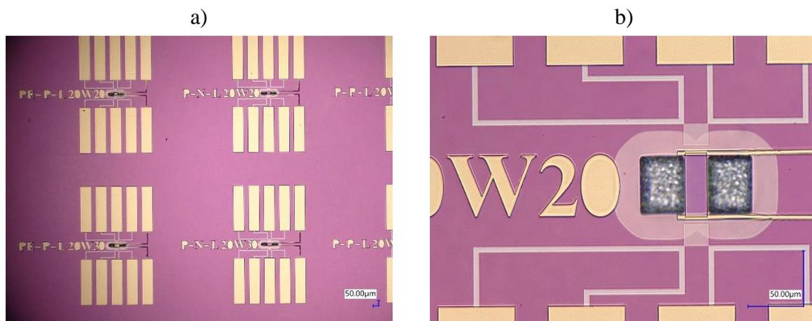
Figure 3: The microscope images showcase a) the fabricated Seebeck coefficient measurement device, b) a close-up view of the Si suspended membrane within the Seebeck coefficient measurement device.
