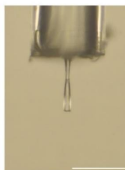
Figure 2. 2. PETA-based tips at the end of SMF-28 obtained by different exposure conditions. The scale bar is 100 \mu\text{m} .
