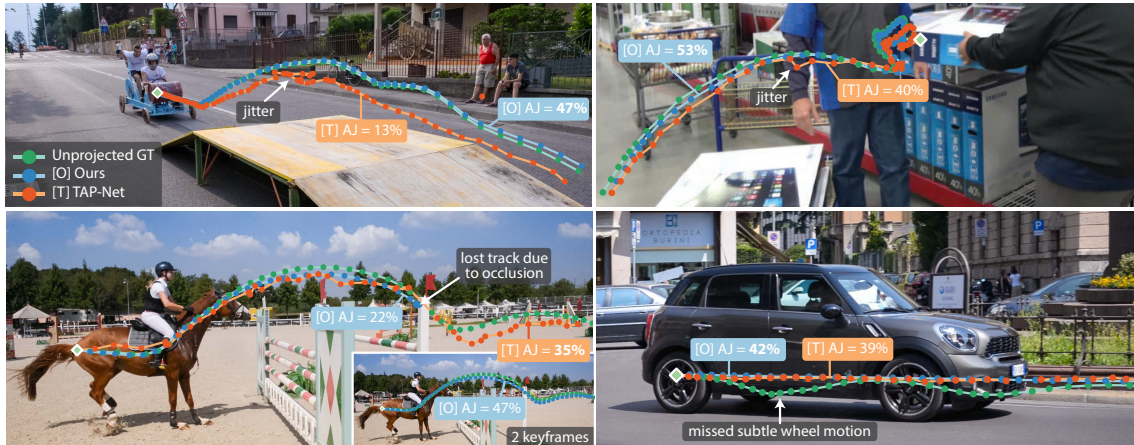
Fig. VI.7: Visual comparison of our tracking trajectories against TAP-Net [83]. For visualization purposes, we compensate for camera motion by rendering 3D trajectories projected onto the first frame of the video clip. Since the ground truth and TAP-Net trajectories are provided as 2D image-space points, we unproject them to 3D using the same cameras and depth maps as used by our method. Our method produces 3D trajectories that are more precise (higher Average Jaccard, AJ) and smoother than TAP-Net (top row). While our method can lose track of a point due to occlusion (bottom left), adding a keyframe often suffices to resolve such issues (inset). Both our method and TAP-Net struggle to recover subtle composed motions, such as the rotation of the car’s wheel (bottom, right).
