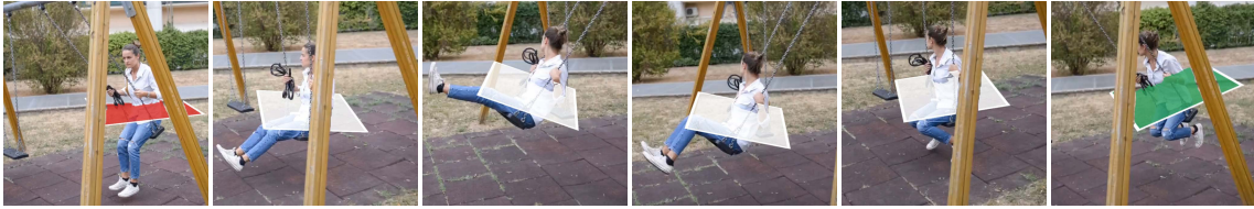
Fig. VI.2: At the core of our interactive system is a novel tracking algorithm that deduces the 3D position and orientation of a planar canvas over an RGBD video given a few keyframes (green denotes a position keyframe, red denotes a position and orientation keyframe). Note how the canvas rotates to align with the direction of the trajectory and gets occluded by the body and the poles. Users create scene-aware doodles by drawing over the canvas in a simple 2D interface.
