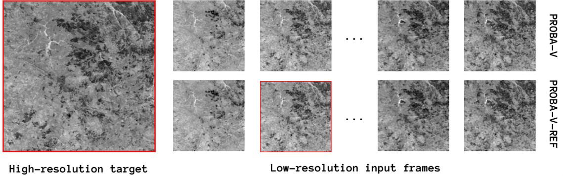
Figure 1.2: The top row presents a LR sequence from the PROBA-V dataset, where the reference frame remains unknown. In contrast, our proposed PROBA-V-REF dataset, shown in the second row, clearly identifies the reference frame, optimizing super-resolution applications.
