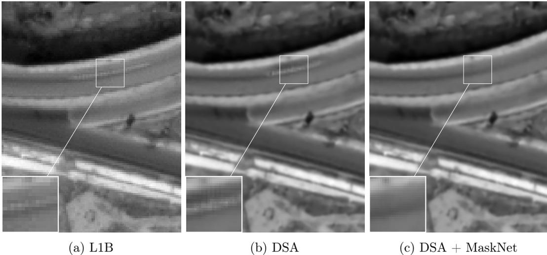
Figure 1.4: Super-resolution from a sequence of 15 real low-resolution SkySat L1A frames. (a) L1B from Planet, (b) DSA, (c) Our improvement with an additional CNN to detect the outliers.
