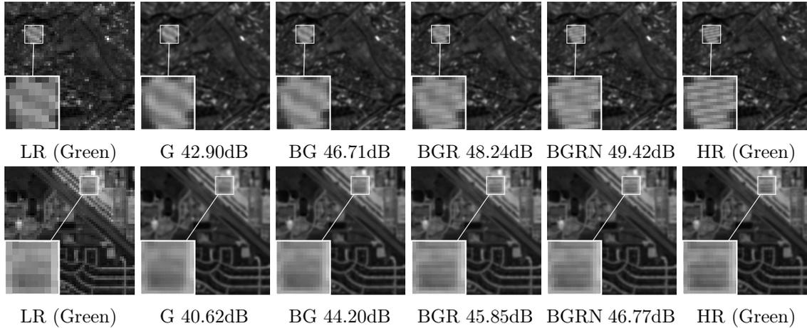
Figure 9.5: SR reconstruction of the green band when trained jointly with different input spectral bands. We observe that the other bands (B, R, N) provide valuable information for improving the reconstruction of the green band.
