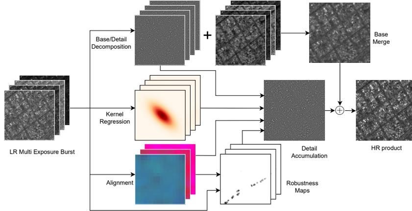
Figure 1.6: An overview of Handheld-SR-Satellite [LNFE23]. In this study, we augment the original handheld burst super-resolution algorithm by [WGDE<sup>+</sup>19] with base-detail decomposition to manage multi-exposure satellite images.
