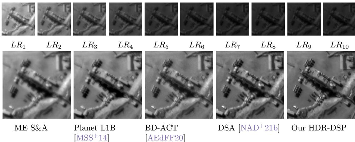
Figure 6.1: Super-resolution from a real multi-exposure sequence of 10 SkySat images. Top row: Original low resolution images with different exposures. Bottom row: Reconstructions from five methods, including ours trained with self-supervision (right).
