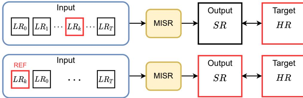
Figure 3.1: The PROBA-V dataset (top) does not make any distinction between the LR images. One of them was acquired at the same time as the target HR image which is used for training and evaluation. The MISR methods need to determine a reference without knowing which is the one corresponding to the target. We propose PROBA-V-REF (bottom), a version of PROBA-V where the identity of true reference is known.
