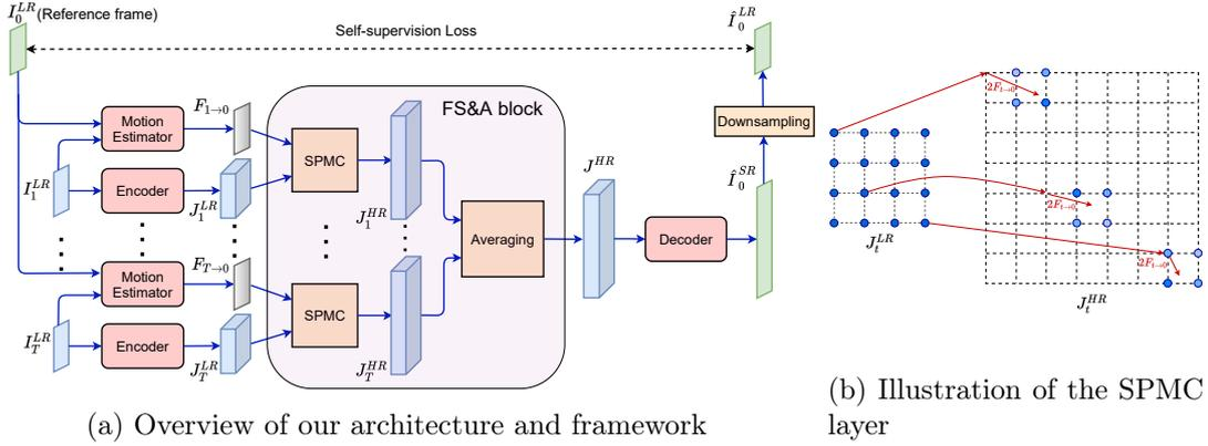
Figure 4.2: (a) Overview of our proposed self-supervised MISR framework at training time. The depicted loss represents the self-supervision term  $\ell_{self}$ , for simplicity the losses concerning the motion estimation module are not illustrated. Note that at inference time the frame  $I_0^{LR}$  is also encoded and fed to the FS&A block. (b) SPMC  $\times 2$  layer [TGL<sup>+</sup>17]: Splating LR features onto the HR domain using the flow  $F_{t \rightarrow 0}$ .
