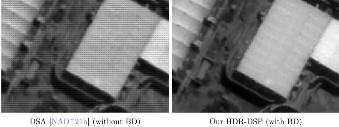
Figure 6.3: High frequency artifacts in a reconstruction from a real SkySat sequence (using DSA [NAD+21b]) with exposure time errors (left). HDR-DSP with the proposed base-detail (BD) decomposition does not present artifacts (right).
