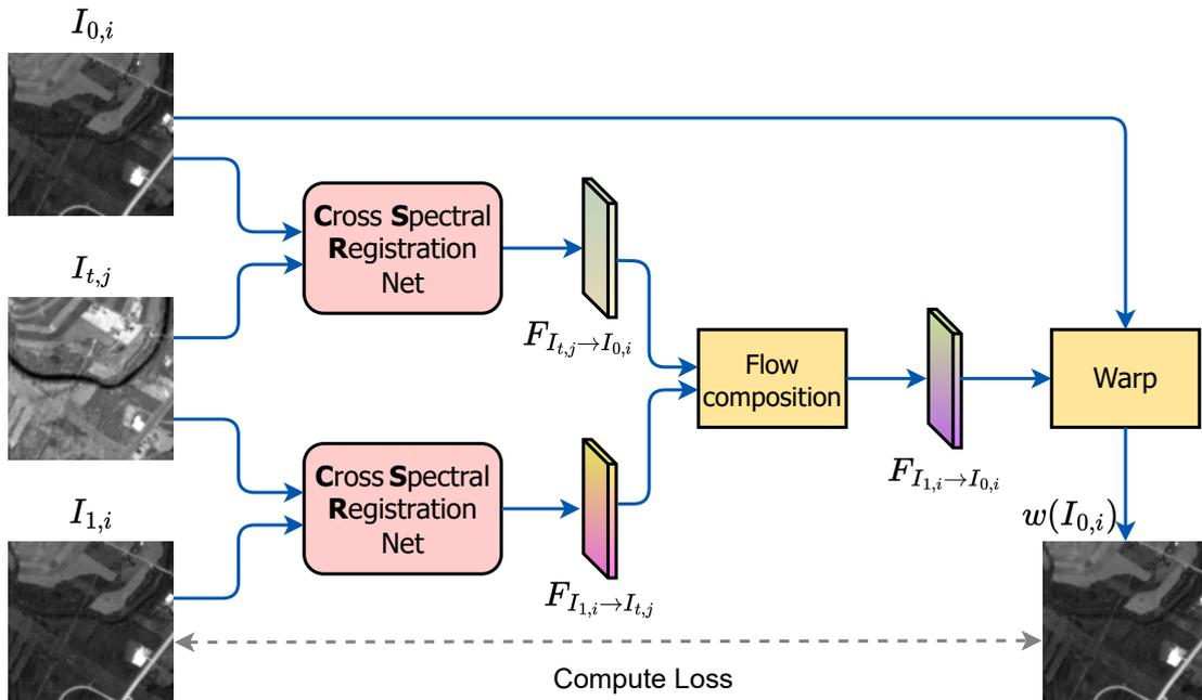
Figure 9.4: Training setup of our proposed cross-spectral registration (CSR) module. The motion from  $I_{0,i}$  to  $I_{1,i}$  via the anchor  $I_{t,j}$  should represent the direct motion between them. The depicted loss represents the Anchor-Consistency loss (9.7).
