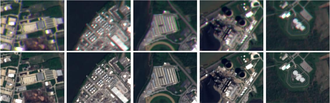
Figure 1.9: L1BSR produces a 5m high-resolution (HR) output with all bands correctly registered from a single 10m low-resolution (LR) Sentinel-2 L1B image with misaligned bands. Note that our method is trained on real data with self-supervision, i.e. without any ground truth HR targets.
