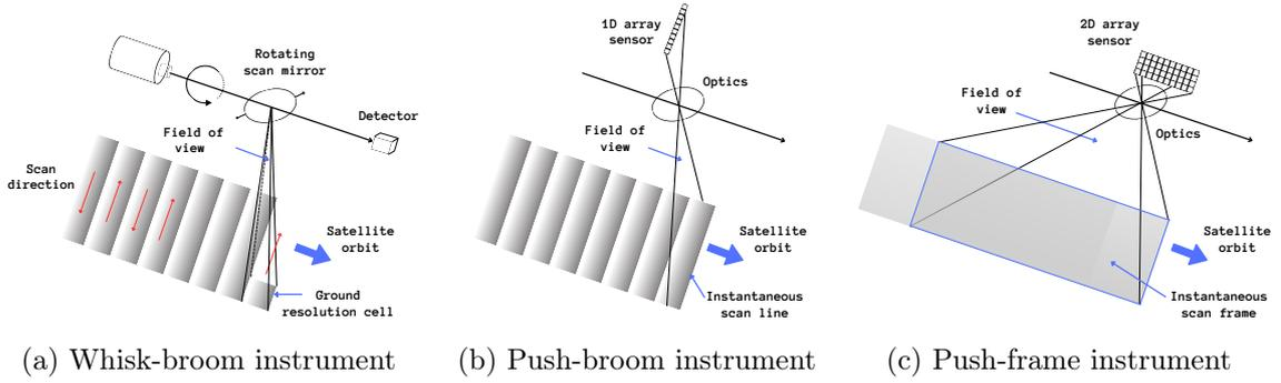
Figure 1.1: A depiction of different satellite imaging technologies, each illustrating the detector of one spectral band: from whisk-broom (1.1a) scanning pixel by pixel through push-broom (1.1b) scanning line by line to push-frame (1.1c) scanning frame by frame.
