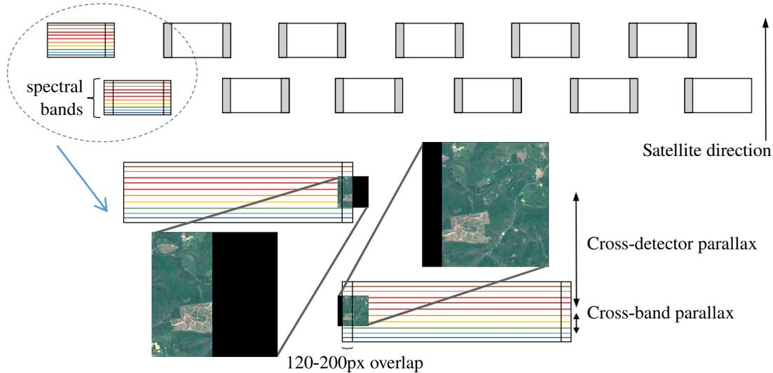
Figure 9.2: Sensor layout of the Sentinel-2 MSI (figure adapted from [GBT<sup>+</sup>17]). The push-broom acquisition is done in the vertical direction. The overlap between detectors provides two near-simultaneous observations of the scene.
