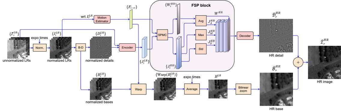
Figure 6.2: Overview of our proposed multi-exposure super-resolution network architecture HDR-DSP at inference time.
