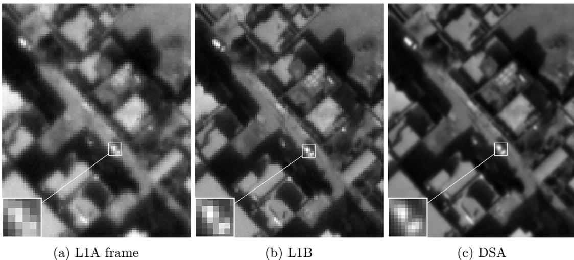
Figure 1.3: Super-resolution from a sequence of 15 real low-resolution SkySat L1A frames. (a) Reference L1A frame, (b) Planet L1B product ( $\times 1.25$ ), (c) Proposed method ( $\times 2$ ).
