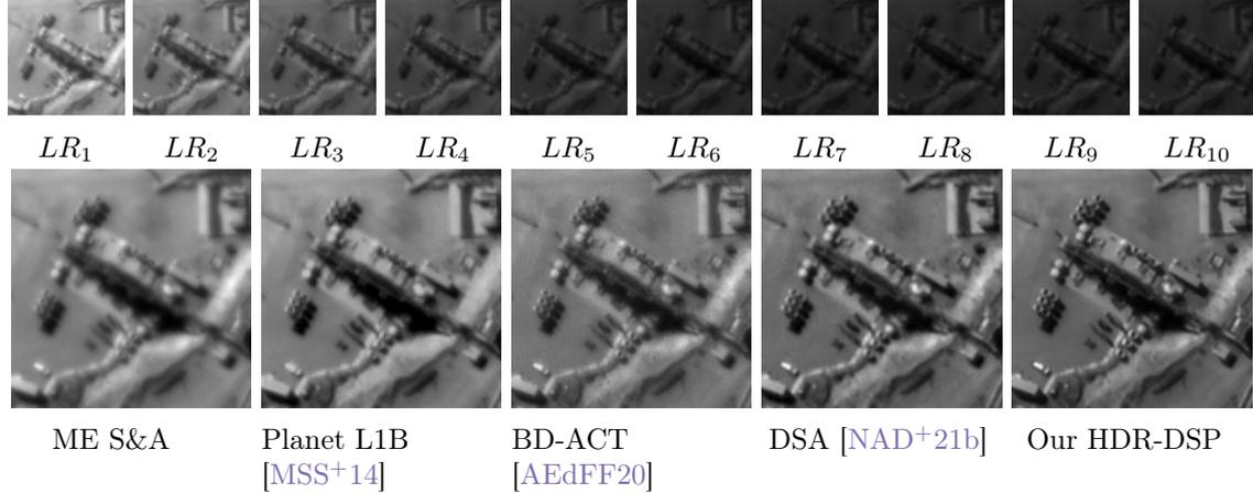
Figure 1.5: Super-resolution from a real multi-exposure sequence of 10 SkySat images. Top row: Bracketed LR sequence. Bottom row: Reconstructions from five methods, including ours trained with self-supervision (right).
