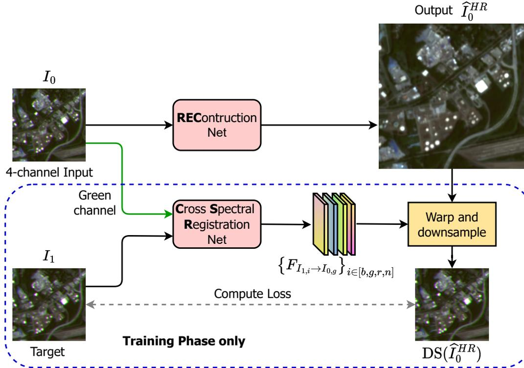
Figure 9.3: Overview of our proposed self-supervised L1BSR framework for Sentinel-2 L1B at training time. The depicted loss represents the self-supervision term  $\ell_{\text{Self-SR}}$  (9.3). Note that at inference time, only one input and the reconstruction module are required.
