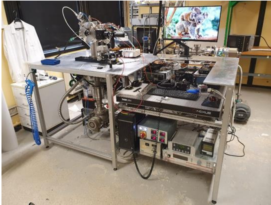
Figure 2-26: Retrofitted PECVD Reactor (left) with in-situ MPL & PL workstation (right).
