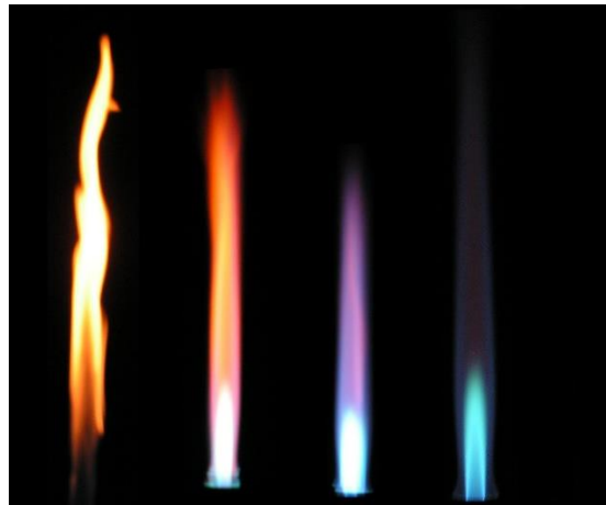
Figure II. 1: Flames of a Bunsen burner with varying premixed oxygen quantities, from the lowest (left), to the highest (right)
