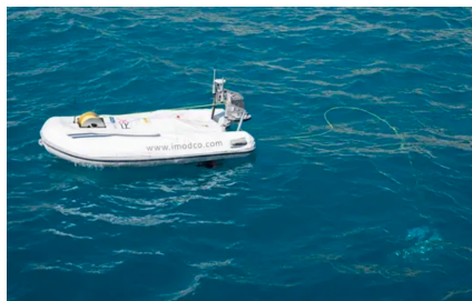
(E) ROV tethered to a USV. Courtesy of IMODCO
