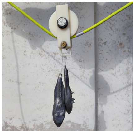
FIGURE 3.20: Sliding ballast composed of a pulley and two masses of 120 g each.
