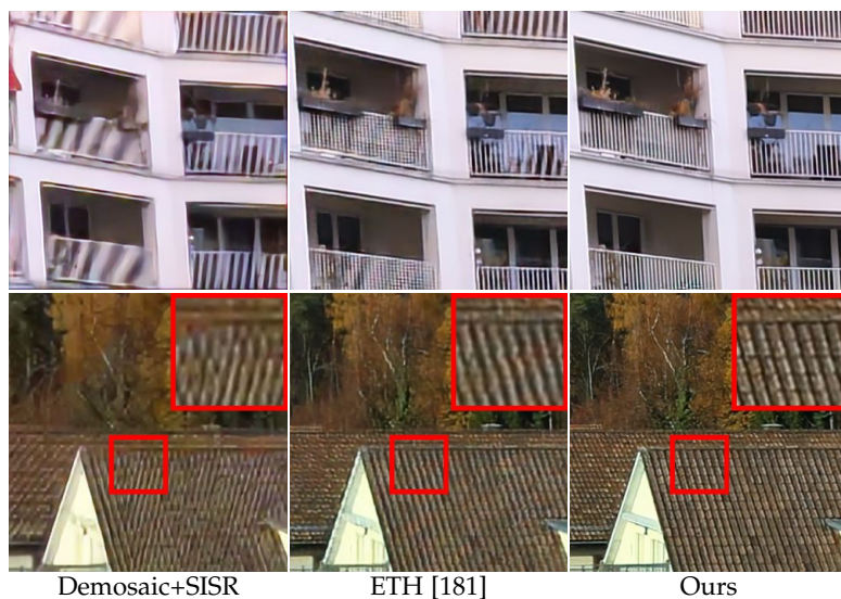
Figure 5.3: Visual comparison on synthetic raw image bursts used in [181]. Demosaic+SISR is our single-image baseline based on the ResUNet architecture [186] (see main text). The two right columns are produced by methods dedicated to raw burst processing, respectively [181] and ours.
