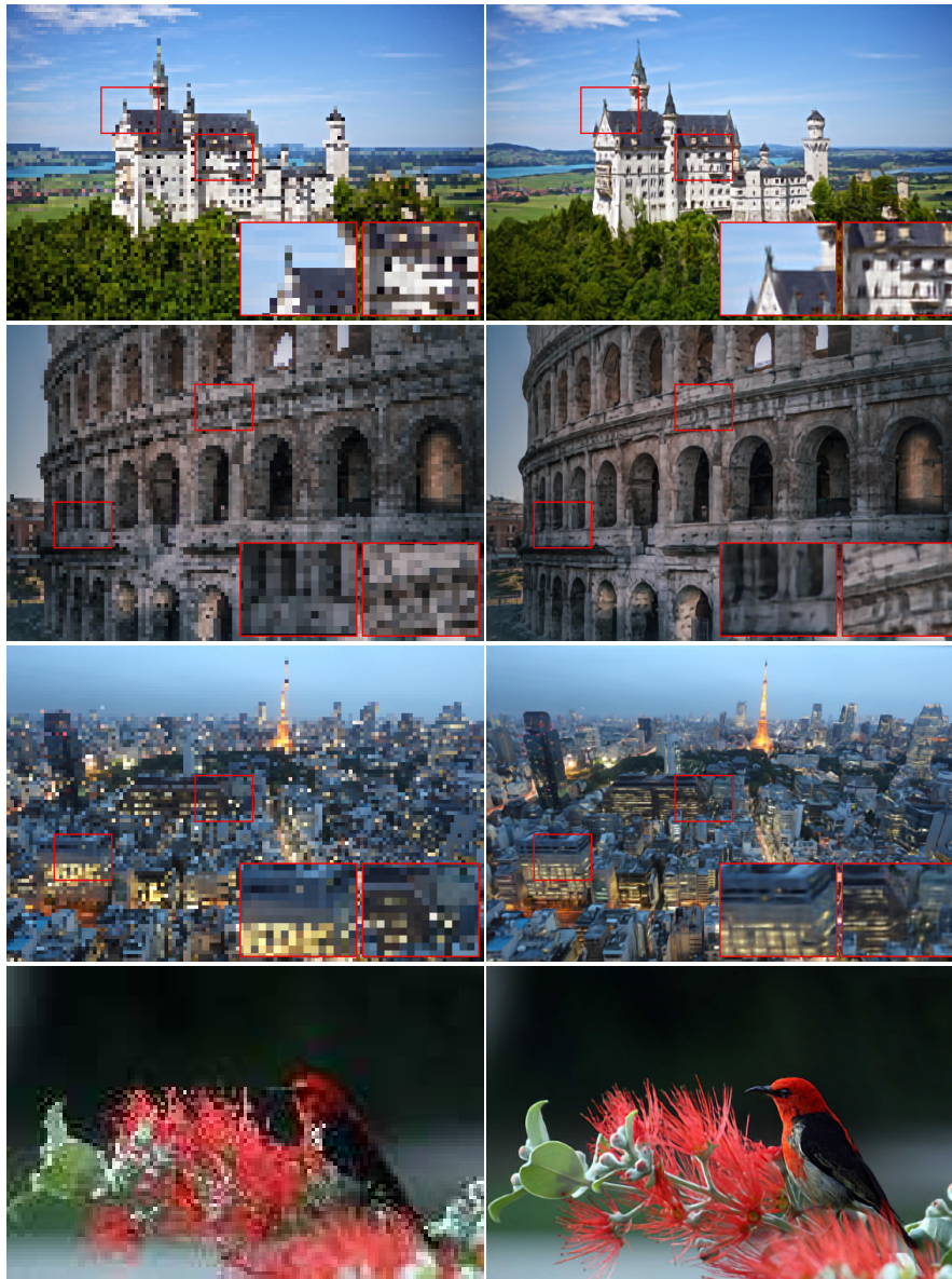
Figure 5.10: Extreme \times 16 upsampling experiment. The right image is obtained by processing a burst of 20 LR images presented on the left obtained with synthetic random affine movements and average pooling downsampling
