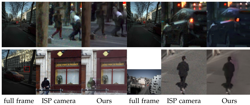
Figure 5.14: Misalignments artefacts due to moving objects in the scene. Our current implementation does not handle fast moving objects and then generates visual artefacts. Dealing with fast dynamic scenes will be the focus of future work.
