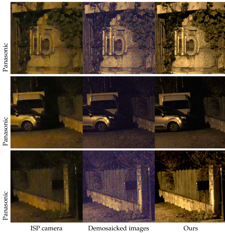
Figure 5.11: Image restoration of images taken at night with very low signal to noise ratio by using a Panasonic GX9 camera.
