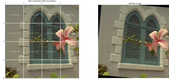
Figure 8.2: Alignment on synthetic data with the hierarchical implementation of the Lucas Kanade. The target image I_1 is synthetically warped with a rotation centered in the middle of the image. The algorithm performs registration on 3 scales and successfully aligns each tile at the finest level. Left: Illustration of each tile and its estimated motion parameters. Right: Warped templated image \mathcal{W}_{\mathbf{p}}I_2 that successfully matches the target image.
