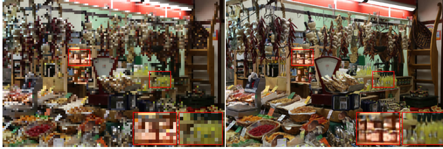
Figure 5.1: Proof of concept for extreme \times 16 upsampling. The right image is obtained by processing a burst of 20 LR images presented on the left obtained with synthetic random affine movements and bilinear downsampling.
