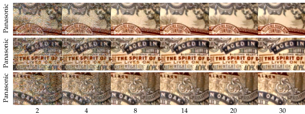
Figure 5.12: Visual differences caused by merging a different number of frames in the case of low SNR scenes. With a larger number of frames we can observe a quality increase and better denoising.
