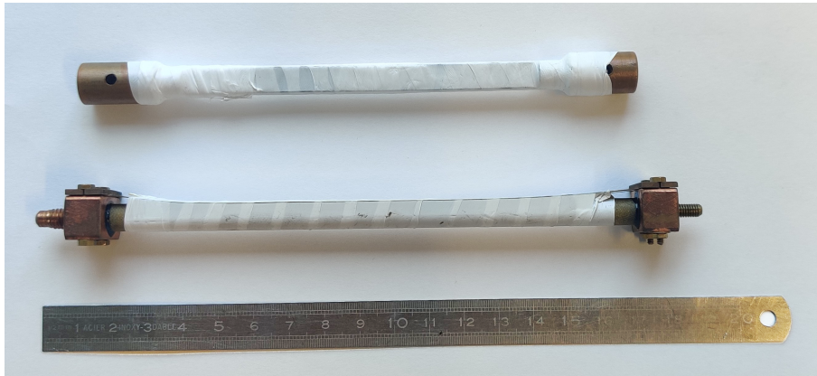
Figure 2.2: Cold fingers ensuring the thermal link between the cold stages of the cryostat and the sample-holder. Top: copper rod. Bottom: fiberglass with a brass strip along its length, held in place by copper pieces, allowing the sample-holder to reach T = 6 K without leaving the dilution regime. Both heat sinks are wrapped in Teflon tape to protect the wires from the sharp edges.
