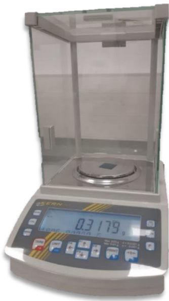
Figure 2.9 Balance Kern AEJ 200-4CM
