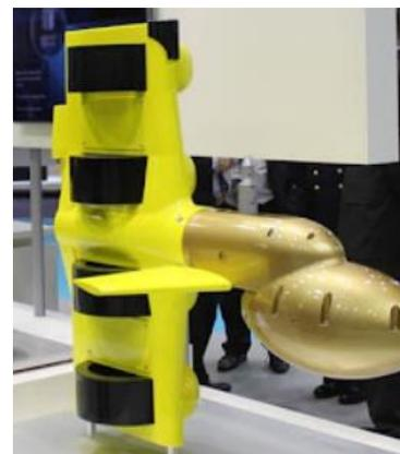
**Figure 2** Sonar CAPTAS 2 (French Navy Mine Warfare & Thales USV for MCM)
