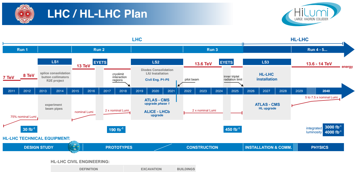
Figure 2.6 LHC baseline plan for the next decade and beyond showing the collision energy (upper line) and instantaneous luminosity (lower line). Plan as taken from Ref. [51] last updated in February 2022.
