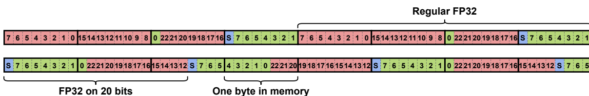
Figure 6.2: Memory representation of 20-bit truncated FP32 data concatenation, along with regular FP32 storage.
